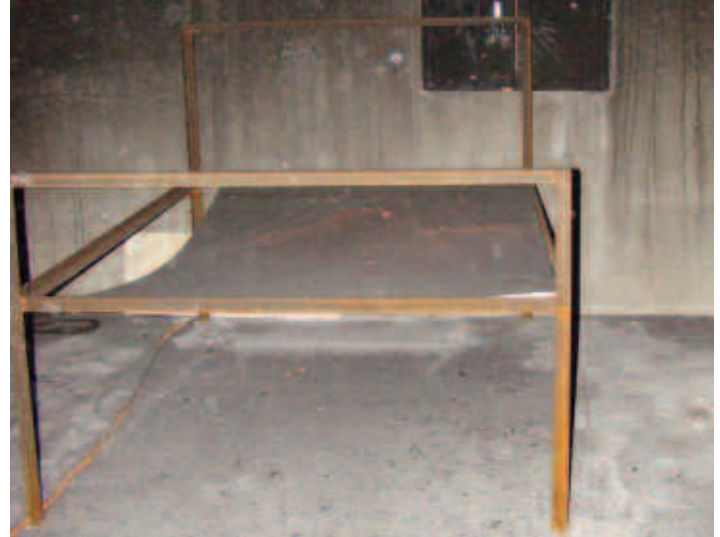
Figure 5: Noncombustible Furniture Used in the Time-to-Task Experiments
