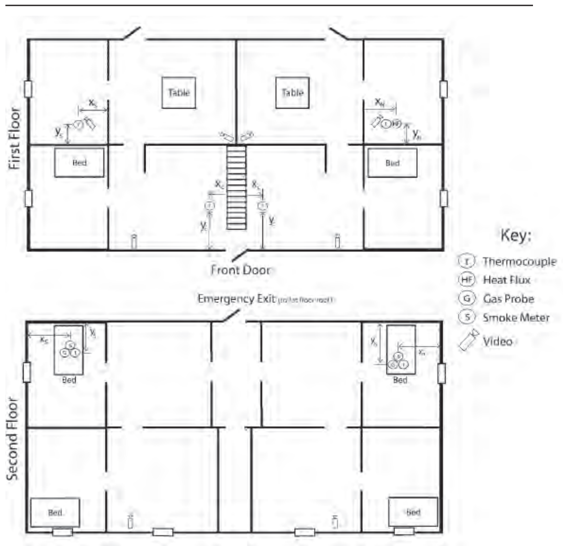
Figure 6: Instrumentation and Furniture Prop Layout
