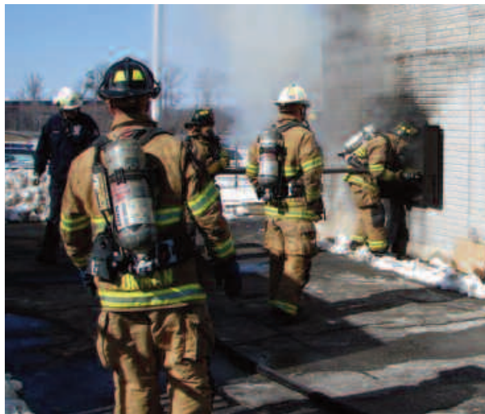
Figure 23: Supplemental Suppression Applied for Room and Contents Tests
